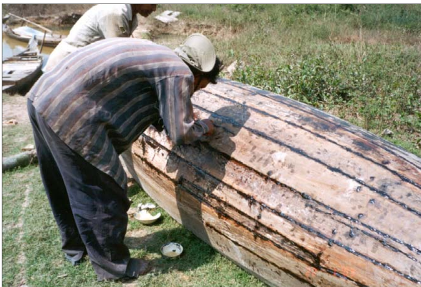
Sealing a fishing boat with resin in Po Village, Kompong Chhnang.
